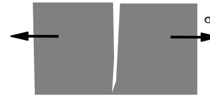
stress corrosion cracking
