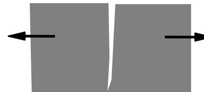
stress corrosion cracking
